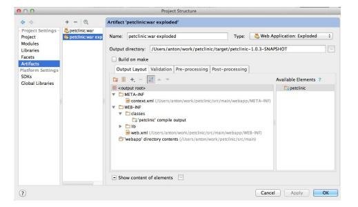
For the "happy-path" scenario, as in our case with the *Petclinic* application, artifacts can be created semi-automatically; you just push the **Fix** button while creating the *Run Configuration*. This is because the sample application makes use of Maven and IDEA integrates well with that.
